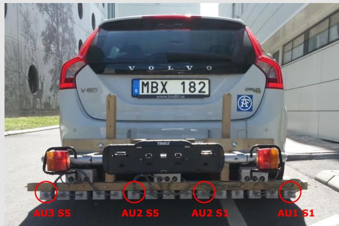
The magnetic field sensor system test rig
